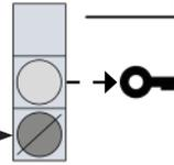
Access key trapped, personnel (safety) key released, access door open.
