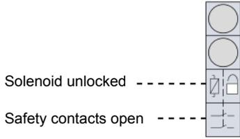
Access keys unlocked, safety contacts open.
